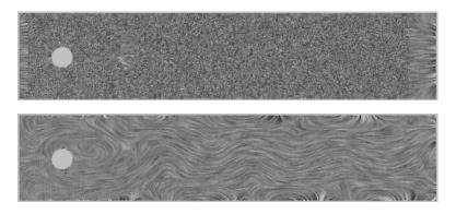
**Fig. 4.** Incompressible flow around a cylinder. Rotation-free component (top) vanishes except at inlet and outlet. Divergence-free component (bottom) has additional artifact at boundary. Courtesy Michael Hinze, TU-Berlin.
