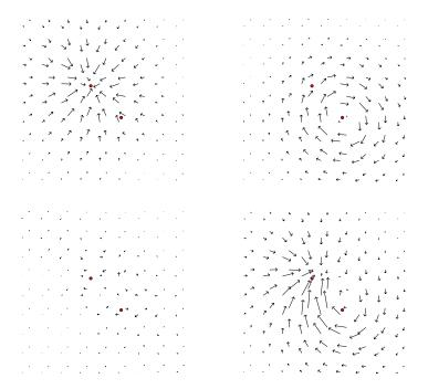
**Fig. 1.** Decomposition of test vector field (bottom right) in rotation-free (upper left), divergence-free (upper right) and harmonic component (bottom left). The two dots in each image indicate the centers of the original potential. Notice, that the dots in the combined vector field do not seem to lie in the centers indicated by the vector field, although they do. But the components clearly recover the original centers. Compare figure 3 for the associated potentials.
