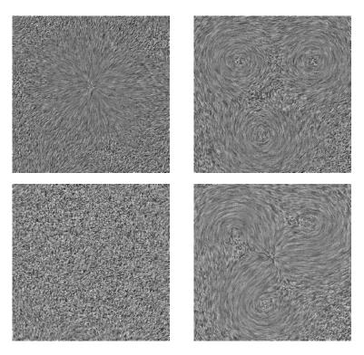
Fig. 2. Test vector field consisting of three vortices and a potential. The algorithm clearly separates the components. The harmonic component (lower left) has only a minor size.
